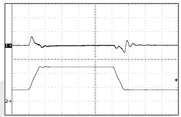
Figure 13: Output voltage response to step-change in input voltage (16 V-50 V-16 V). Load cap: 10 μF, 100 mΩ ESR tantalum cap and 1 μF ceramic cap. Ch 1: Vout (200 mV/div). Ch 2: Vin (20 V/div). Horizontal Timescale: 200 μsec/div.
