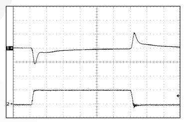
Figure 12: Output voltage response to step-change in load current 0%-50%-0% of Iout (max). Load cap:  $1 \mu F$  ceramic cap and  $10 \mu F$ ,  $100 \, m\Omega$  ESR tantalum cap. Ch 1: Vout (200 mV/div). Ch 2: Iout (10 A/div). Horizontal Timescale:  $100 \, \mu sec/div$ .
