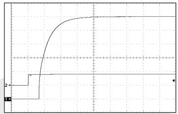
Figure 7: Turn-on transient at full resistive load and zero output capacitance initiated by ENA1. Input voltage pre-applied. Ch 1: Vout (1 V/div). Ch 2: ENA1 (5 V/div). Horizontal Timescale: 5 msec/div.
