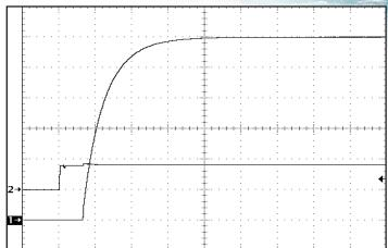
Figure 8: Turn-on transient at full resistive load and 10 mF output capacitance initiated by ENA1. Input voltage pre-applied. Ch 1: Vout (1 V/div). Ch 2: ENA1 (5 V/div). Horizontal Timescale: 5 msec/div.
