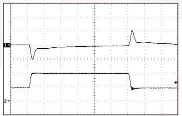
Figure 11: Output voltage response to step-change in load current 50%-100%-50% of Iout (max). Load cap: 1  $\mu$ F ceramic cap and 10  $\mu$ F, 100 m $\Omega$  ESR tantalum cap. Ch 1: Vout (300 mV/div). Ch 2: Iout (10 A/div). Horizontal Timescale: 100  $\mu$ sec/
